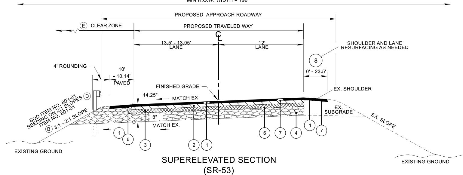
(BASED ON STD. DWG. RD11-TS-3) FROM STA. 21+18.32 TO STA. 21+52.84 (10' LT SHLDR, 13.5' LT LANE, & 11' RT LANE) FROM STA. 21+52.84 TO STA. 22+41.72 (TRANS. 10' TO 10.14' LT SHLDR, 13.5' TO 13.05' LT LANE, COLD PLANE AND RESURFACE RT LANE)
