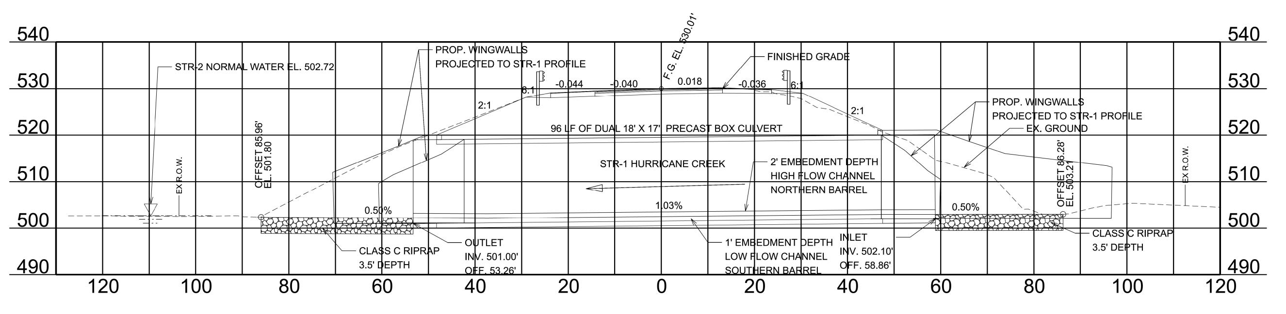
CROSS SECTION FOLLOWS LOW FLOW CHANNEL & STR-1 CENTERLINE
